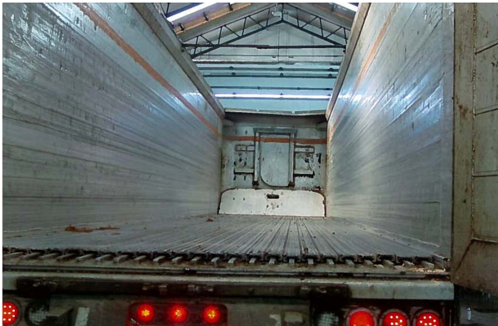
Figure 2 – Trailer's movable floor unloading system.
