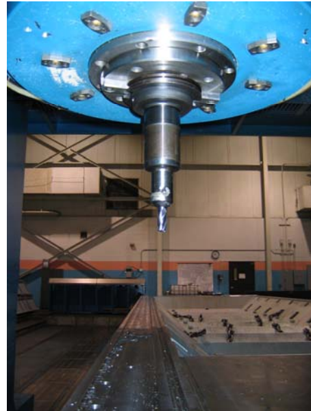
Figure 1. Cutting head of vertical gantry mill and part being machined
