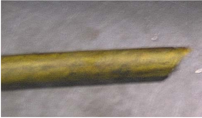
Figure 2. Picture of severed air hose
