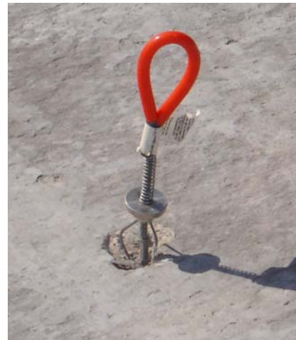
Figure 3. Life line anchor for fall protection lanyard
