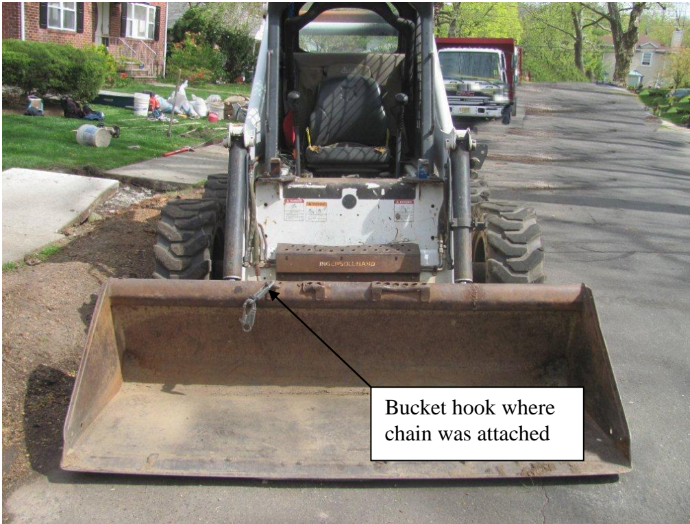
FIGURE 4. Skid-steer loader; note bucket hook where chain was connected.
