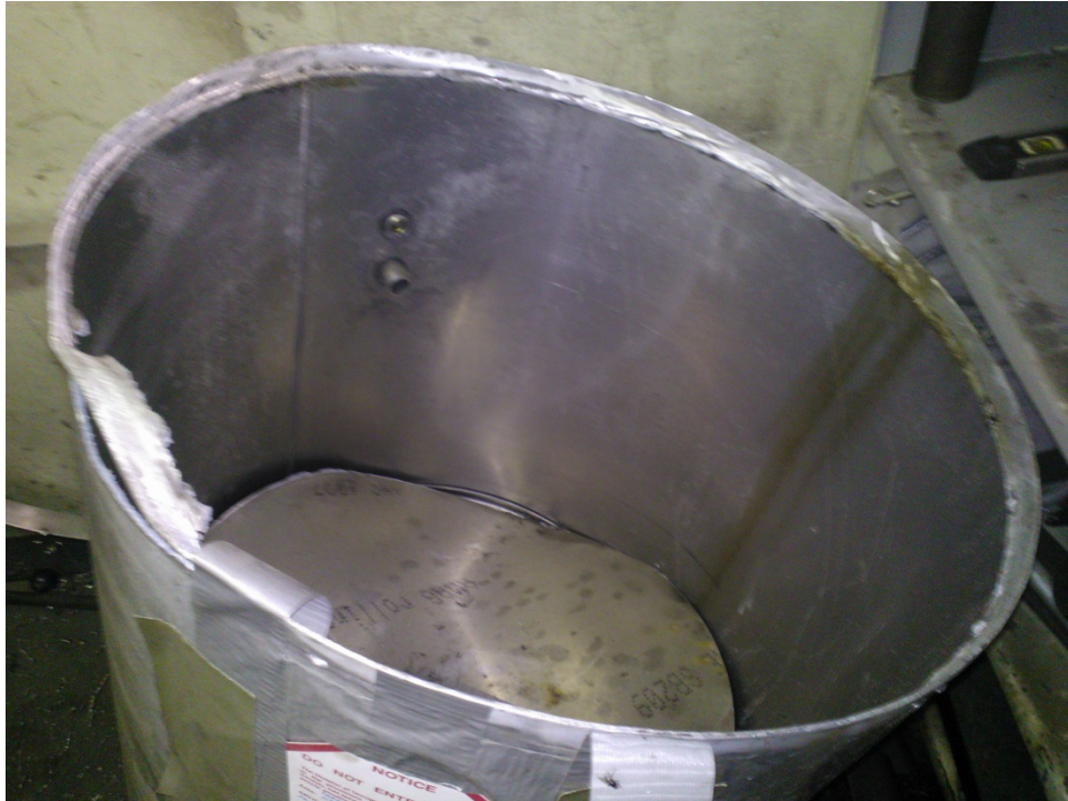
Exhibit 4. The portion of the hydraulic tank that came off under air pressure.
