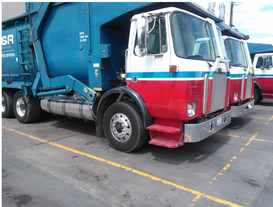
Exhibit 1. A waste collection vehicle with fuel and hydraulic tank similar to the one involved in the incident.
