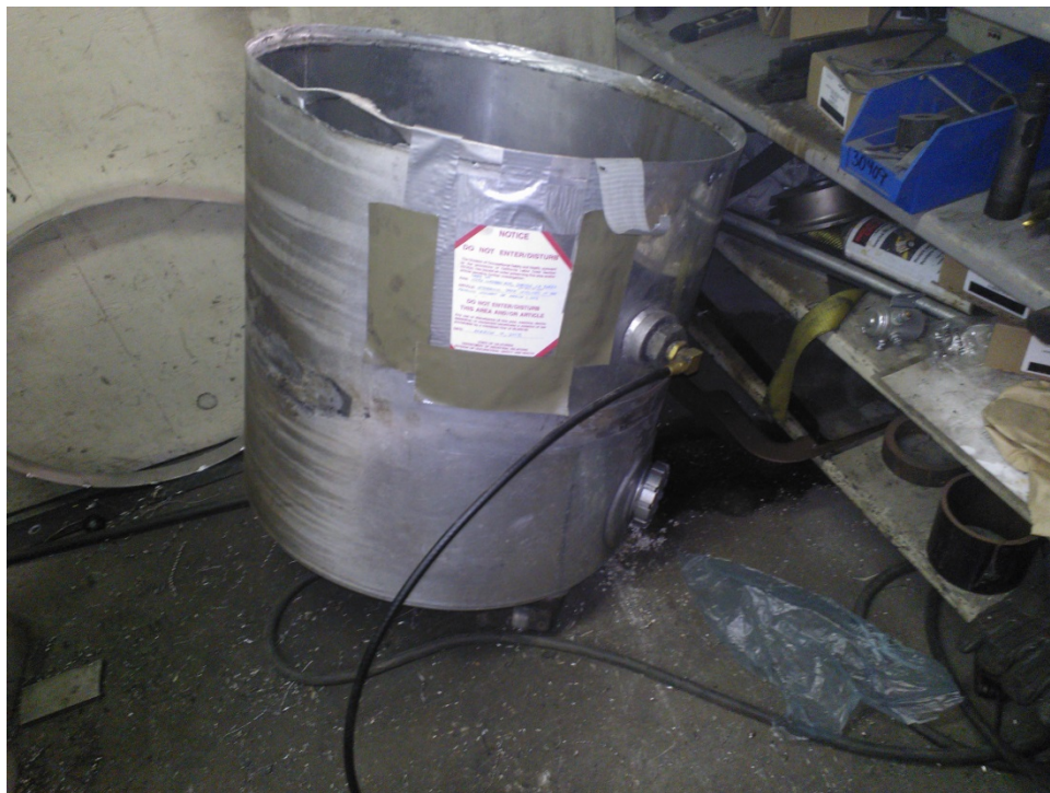
Exhibit 3. The hydraulic tank involved in the incident.
