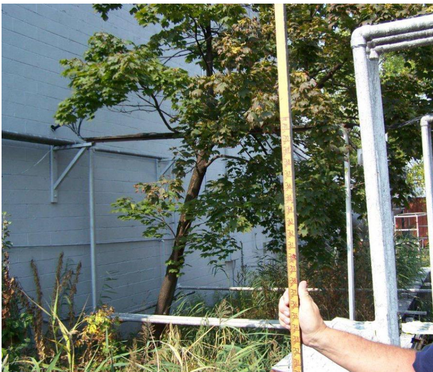
Figure 3. Eighty-four-inch-long wooden measuring stick used to manually gauge the volume of the remaining liquid in the tank.
