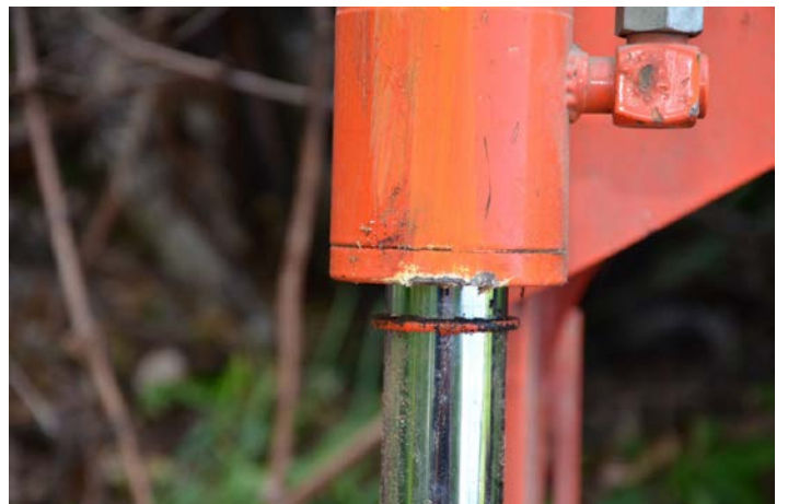
Photo 9. Marks on hydraulic arm/cylinder caused by tree
