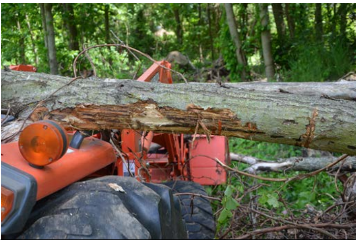
Photo 6. Marks on tree caused by loader bucket and hydraulic arms from multiple attempts to push tree
