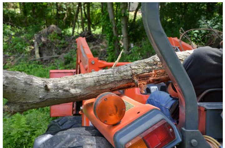
Photo 7. Marks on tree caused by loader bucket and hydraulic arms from multiple attempts to push tree
