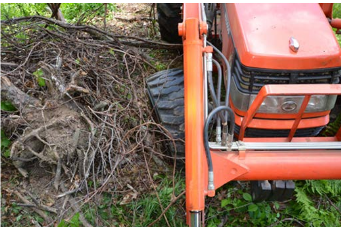
Photo 8. Paint transfer marks on hydraulic arm caused by tree
