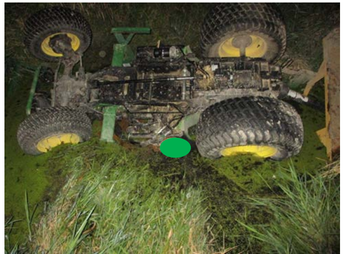
Photo 4. Overturned tractor in the ditch. Green oval is location of decedent under the tractor.
