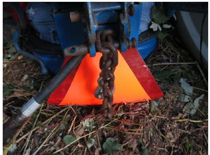
Photo 5. Location of chain on tractor and SMV sign placement/orientation at time of incident
