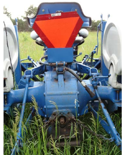
Photo 3. Placement of SMV sign behind tractor seat and no drawbar
