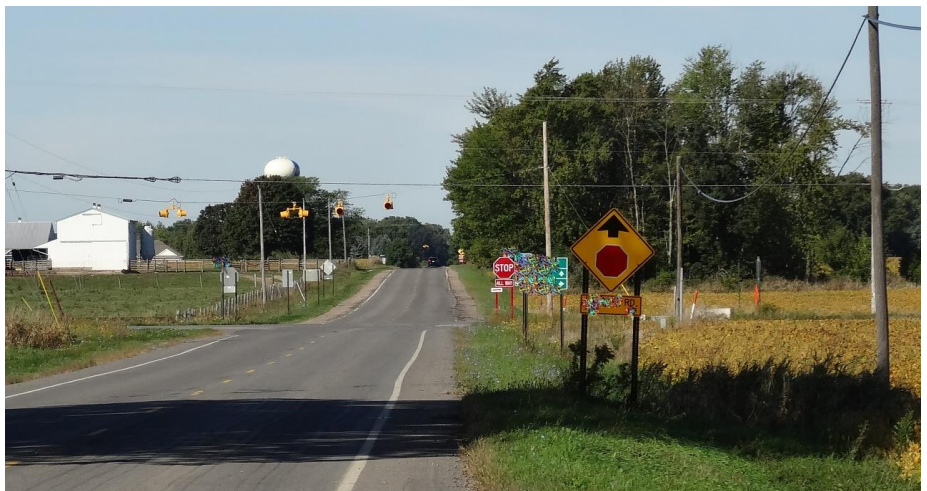
Photo 4. Flashing red light installed, 4-way stop indicated at intersection stop sign
