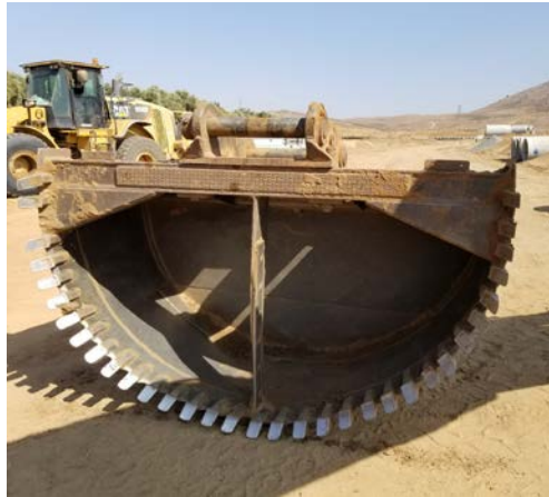
Exhibit 4. The bucket that disconnected from the coupling.
