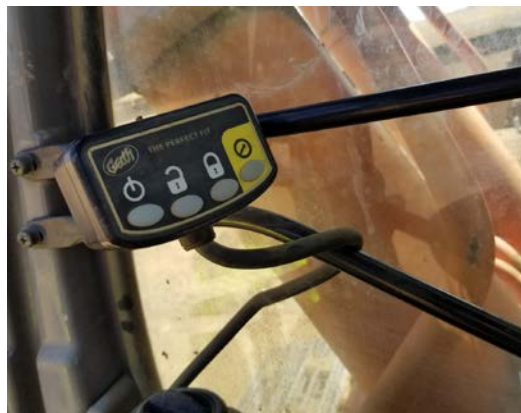
Exhibit 3. The automatic hydraulic quick coupler control panel.
