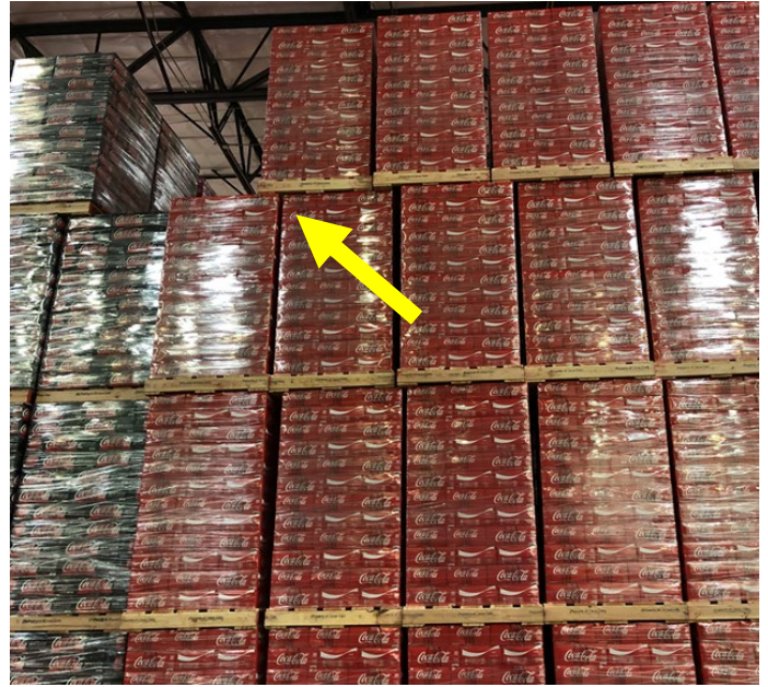
Image 3. Back of pallet row. Note offset of top (4th) pallet layer overhangs rear edge of 3rd layer (yellow arrow). Also note back of pallet row abuts back of adjoining pallet row containing a different product.
