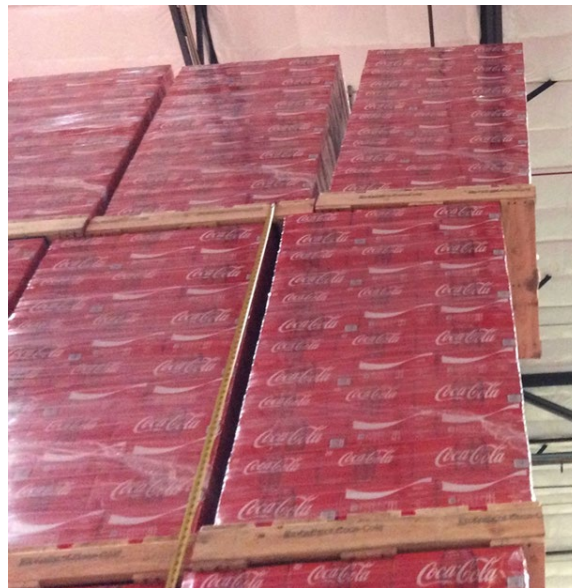
Image 4. Side view of end of pallet row where incident occurred. Top (4 th ) pallet layer overhanging 3 rd layer and leaning away from top pallet row. The pallet next to this leaning pallet was the one that fell on the decedent.
