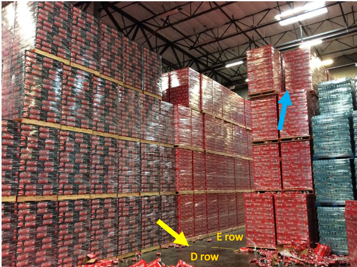
Image 5. Looking at front of D row and the back of E row. Note 1: The faded yellow line on the floor that marks the end of one pallet row and the beginning of another (yellow arrow). Note 2: The pallets at the end of E row do not have pallet labels on
