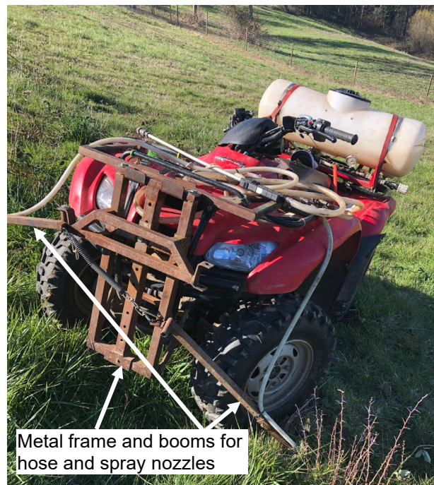
Image 3. Front view of ATV modified with herbicide sprayer apparatus.
