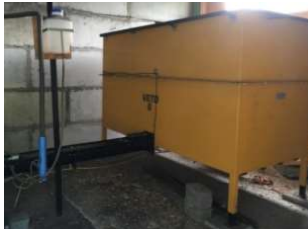
Figure 2 - The hopper and wood chip auger/conveyor
