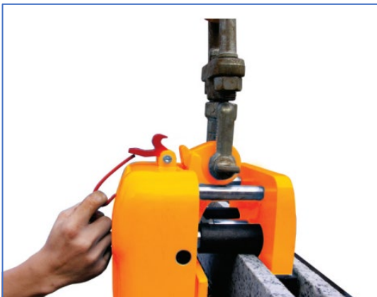
Photo 8. Unlocking of Latch of Lifting Device [ABACO Machines]
