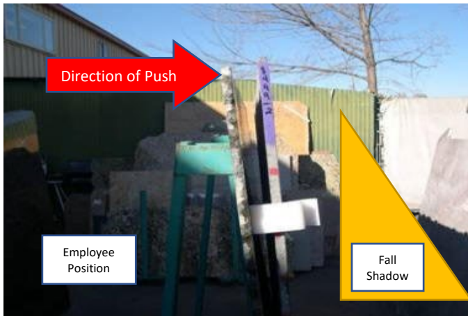
Photo 7: Positioning Relative to Rack [OSHA 2008]
