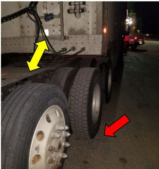
Photo 13: Red arrow in top left photo shows approximately where the driver's body was found crushed under the chip truck's left front drive wheels. Yellow arrows show base of front trailer ladder and walkway between cab and trailer that the driver attempted to access as his truck rolled.
