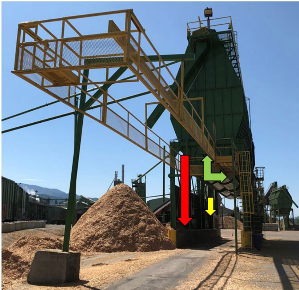
Photo 10: Red arrow shows where the back of the fatally injured driver's trailer was aligned under the back of the tarping station above. Green arrows show the ladder and platform that allowed the driver to access the rear top of his trailer. Yellow arrow shows where the front of the second truck's tractor was located under the bins when the incident occurred. Approximately 30 feet of space separated the trucks. The paved road under the tarping station had a 2% downgrade toward the exit in the foreground.
