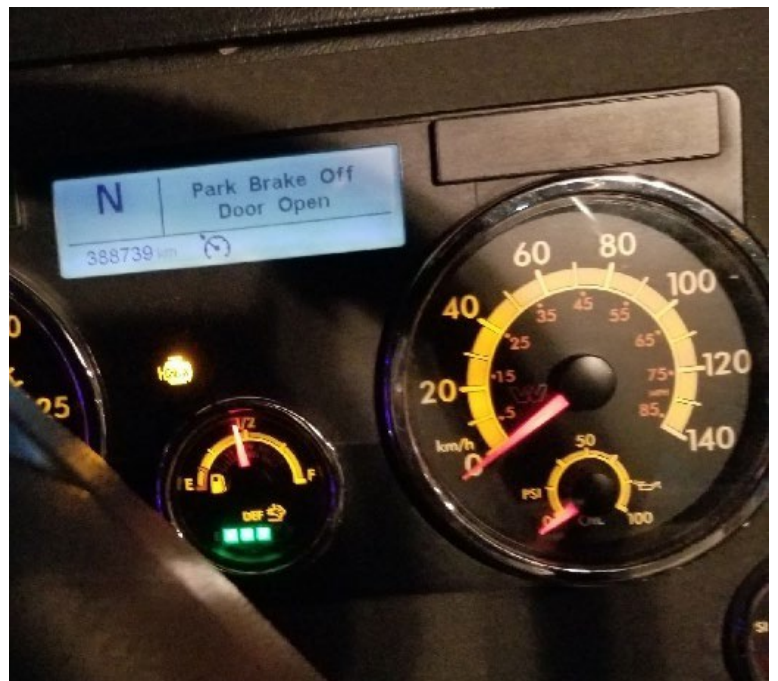
Photos 14 and 15: Bottom left photo shows chip truck's transmission shifter set to "N" neutral after the crushed driver was found. The transmission did not have a "P" park position. Bottom right photo shows dashboard instrument panel indicator showing that the truck's transmission shifter was in "N" neutral and parking brake disengaged when the incident occurred.
