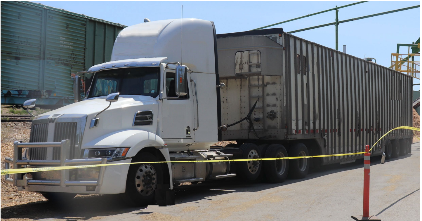
Photo 1: The fatally injured driver operated this 2016 Western Star semi-tractor with a 2004 TYCROP high-cube, quad-axle, possum belly Super B-train chip trailer.
