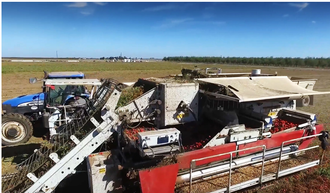
Exhibit 3. Close-up of a tomato harvester during the harvesting process. Photo courtesy Westside Equipment.
