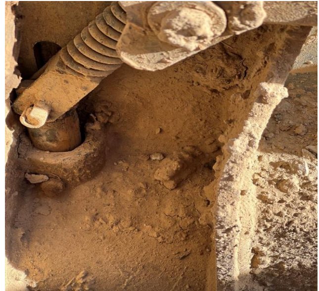
Photo 8. Detail of locking pin (Courtesy of KY FACE).
