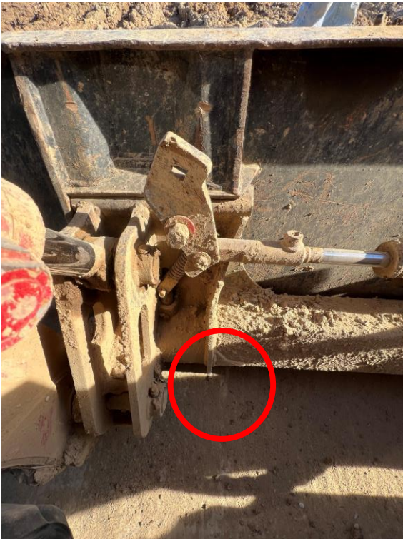
Photo 7. Skid-steer locking pin (Courtesy of KY FACE).
