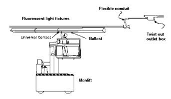
Figure. Worker Replacing Ballast from Manlift Platform
