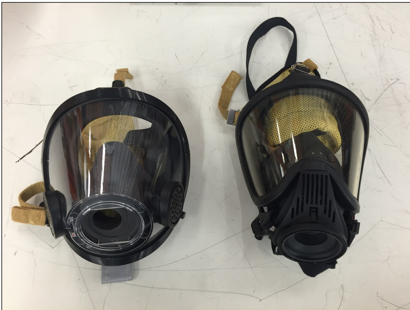
Photo 3. Photo for representative purposes only. Facepiece on the left is representative of the SCBA facepieces used by Department 41. The facepiece on the right is representative of the SCBA facepieces used by Department 19. The Department 41 lieutenant was using a facepiece similar to the one on the right during the incident. (NIOSH photo.)
