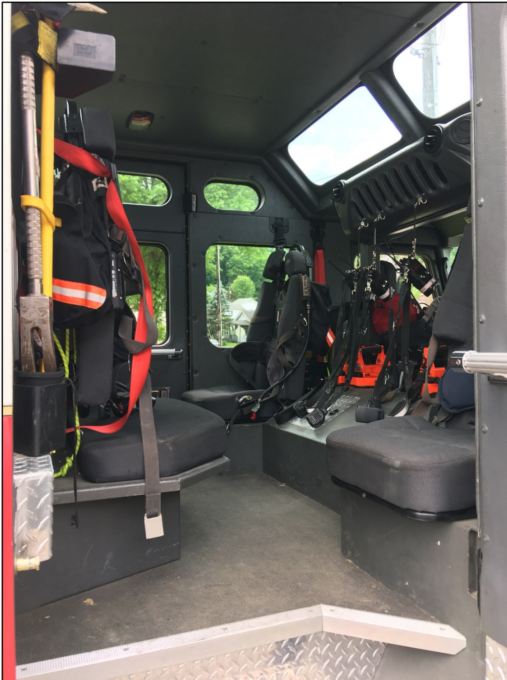
Photo 3. The layout of the jumpseats of Rescue 111 from the passenger side of the apparatus. Note: This photo was taken of a cab of a similar 2004 Typhoon pumper. (NIOSH Photo.)
