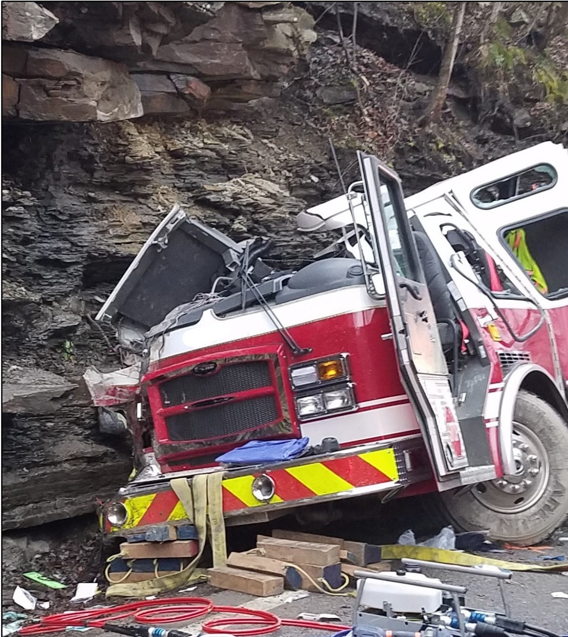
Photo 6. This photograph was taken after the extrication of the fire fighter that was pinned against the rock outcrop and Rescue 111. None of the damage to Rescue 111 was done by the extrication process.
