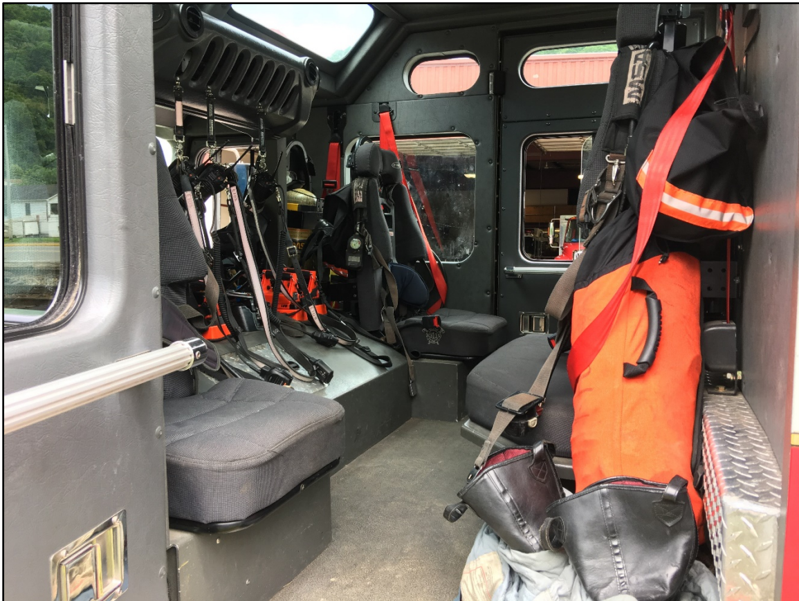
Photo 4. The layout of the jumpseats of Rescue 111 from the driver's side of the apparatus. Note: This photo was taken of a cab of a similar 2004 Typhoon pumper. (NIOSH Photo.)
