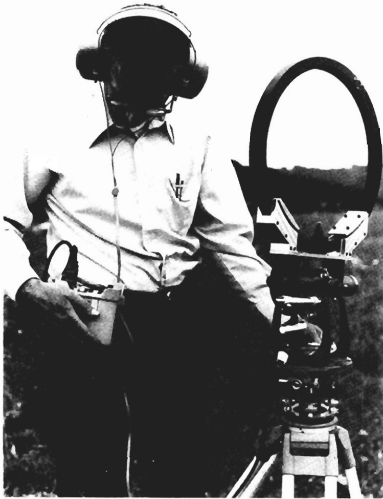
FIGURE 6. - Receiver coil mounted on transit.
