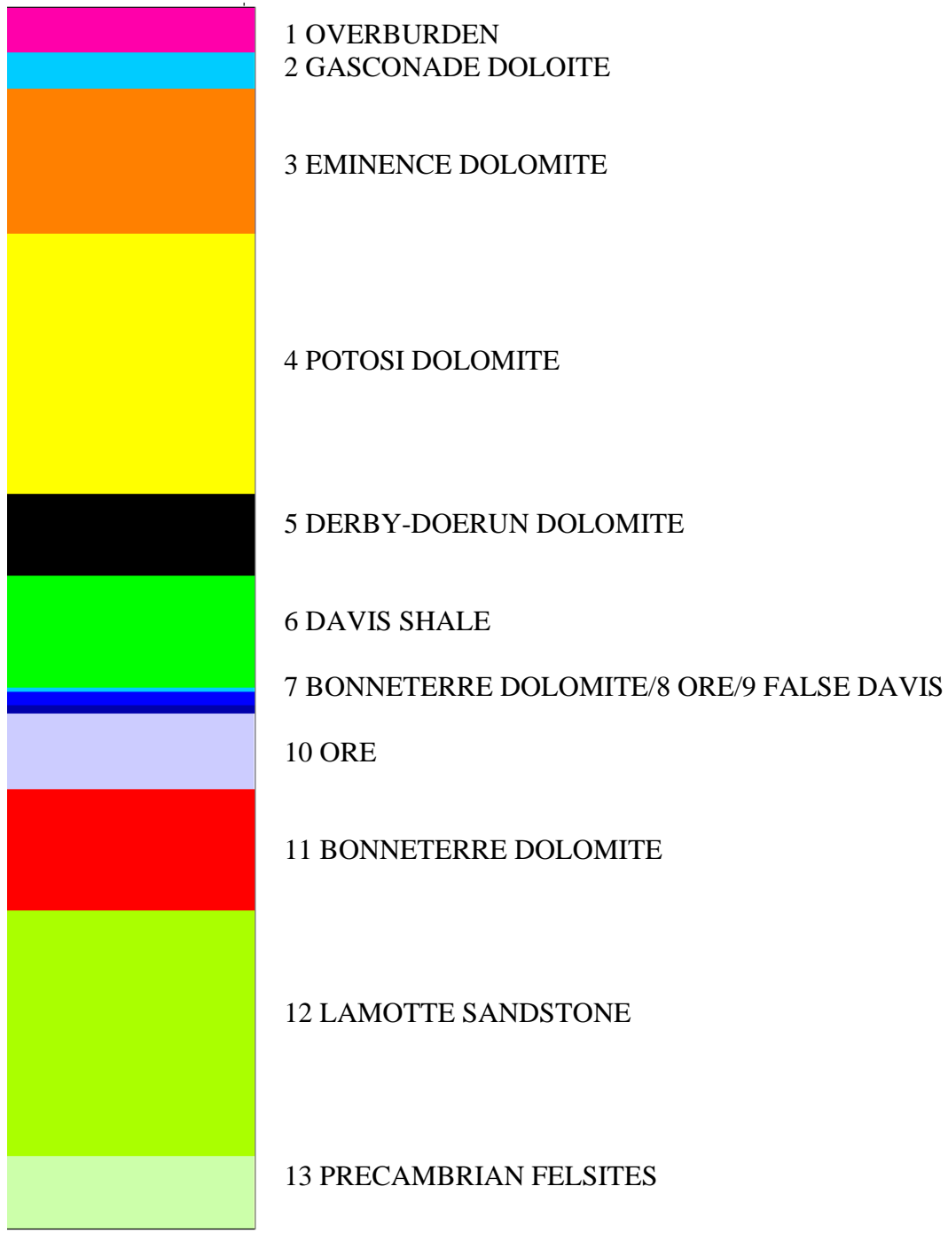
Figure 14 Stratigraphic column for example problems. Pillar is in Unit 10.
