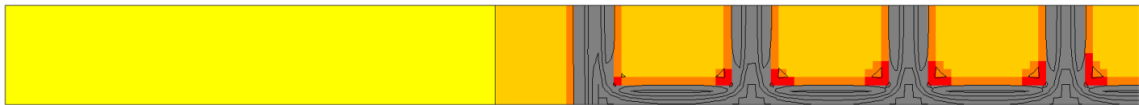
(a) Plan view of element safety factor distribution at pillar mid-height without joints
