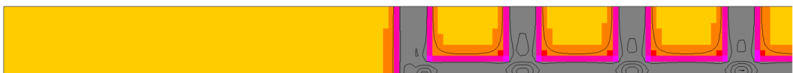
(c) Plan view of element safety factor distribution at pillar mid-height using equivalent properties
