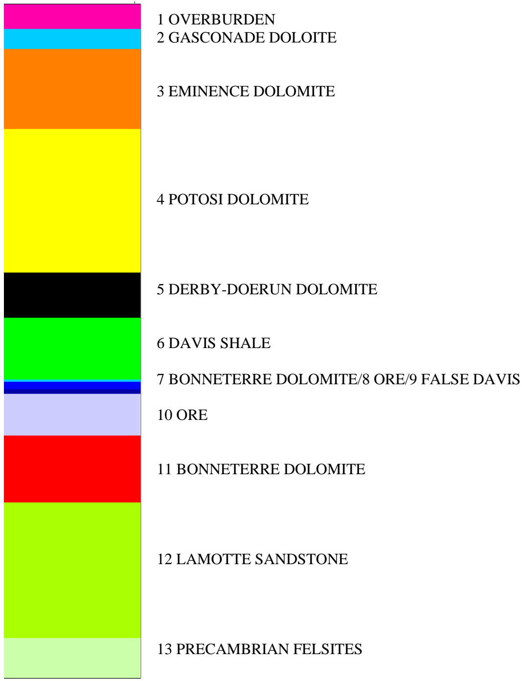
Figure 57 Stratigraphic column for example problems. Pillar is in Unit 10.
