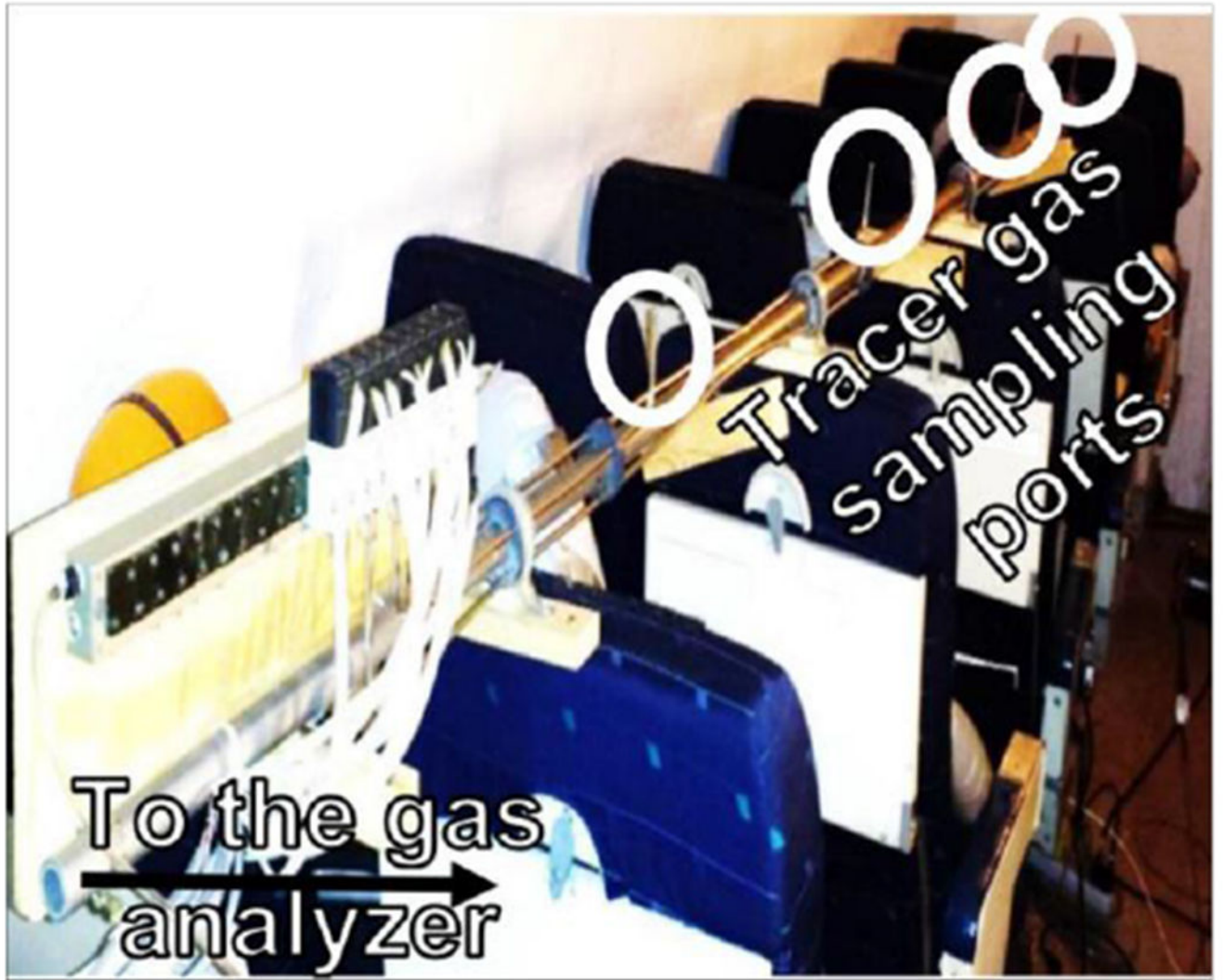
Figure 5. Tracer gas sampling tree. Vertical copper sampling tubes are indicated by white circles. The pneumatic controller is shown on the left.
