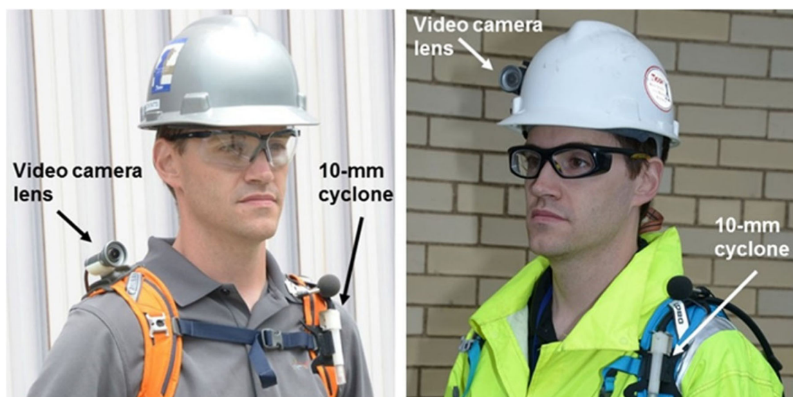
Fig. 2. Helmet-CAM with video camera lens located on worker's shoulder (left) and helmet (right) and the 10-mm cyclone attached to the backpack shoulder harness
