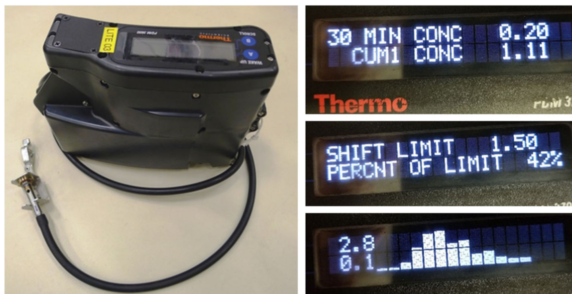
Fig. 4. PDM 3700 dust monitor (left) and information screens available (right). The screen view shown in the top right photo in Fig. 4 provides the average respirable dust concentration for the previous 30 min of sampling, in addition to the average cumulative concentration from the beginning of the sampling shift. The screen shown in the middle right photo identifies the PEL for the sampling shift (input by the user) and the percent of this limit that has been reached to this point of sampling. The last screen photo shows a bar graph of average dust concentrations for each 30-min period of sampling throughout the shift with the values of the highest and lowest measured mass concentrations also displayed
