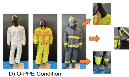
Figure 1. PPE ensembles, with varying interface control measures, worn with cotton long-sleeve base layers: A) standard (S-PPE) B) interface control (I-PPE) C) enhanced interface control (E-PPE) and D) one-piece liner (O-PPE).
