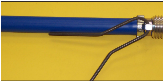
Figure 8. Safety spring hanger installed in the deepest anchor
