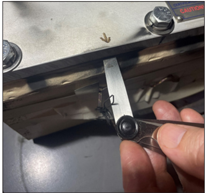
Figure 10. A 0.004-inch feeler gauge penetrated the cover joint in several places after the thermal runaway test
