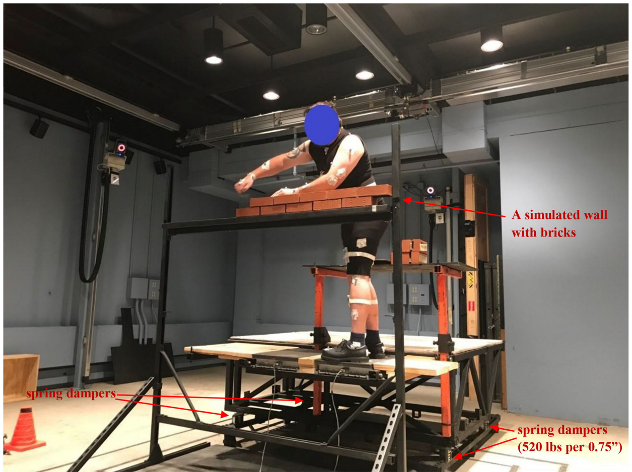
Figure 1. A mason worker performing the simulated bricklaying task on the workstation equipped with the manufacturer straight-shaped production table and simulated wall
