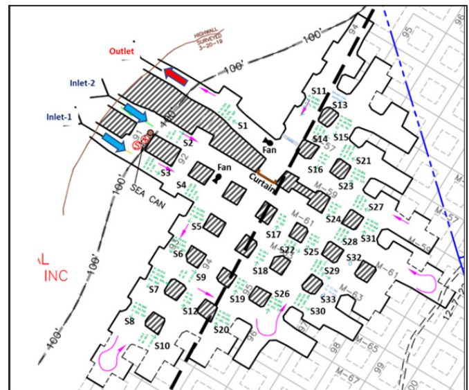
Figure 1. Mine layout showing ventilation control and stations of first ventilation survey (S1–S33)
