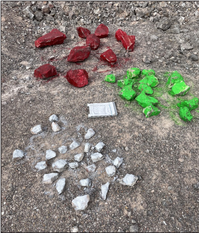
Figure 3. Example of local rocks collected and spray painted prior to rockfall testing
