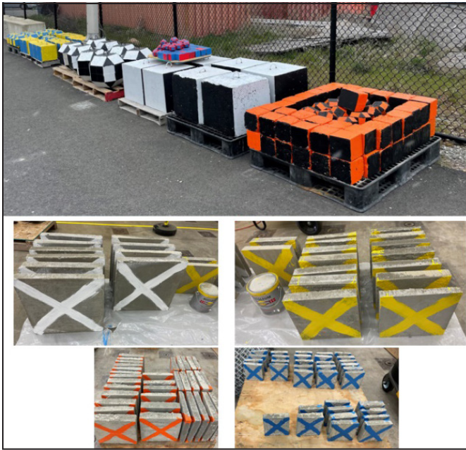
Figure 2. Completed and demolded synthetic rocks colored to distinguish size and shape during post-test analysis.
