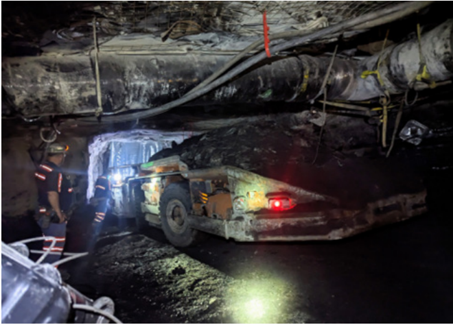
Figure 17. Example of a mine employee making positive contact with a shuttle car operator to inform them of additional employees and researchers working in the area
