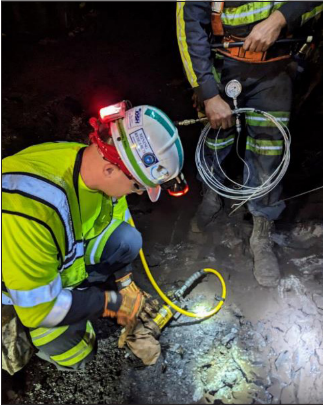
Figure 8. Photo of a researcher pressurizing the BPC to its initial setting pressure using a hydraulic pump
