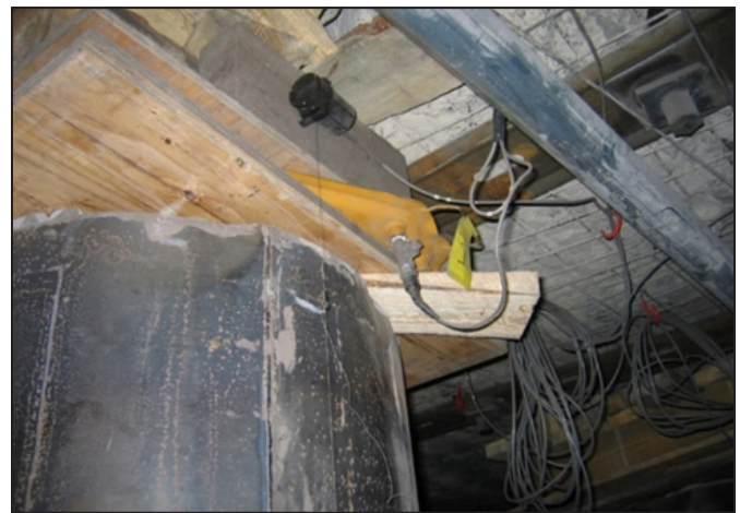
Figure 12. An example of a standing-support load cell installed on top of a can type standing support between two sheets of plywood.
