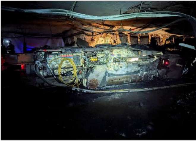
Figure 2. Example of tramping a continuous miner representing a potential struck-by hazard
