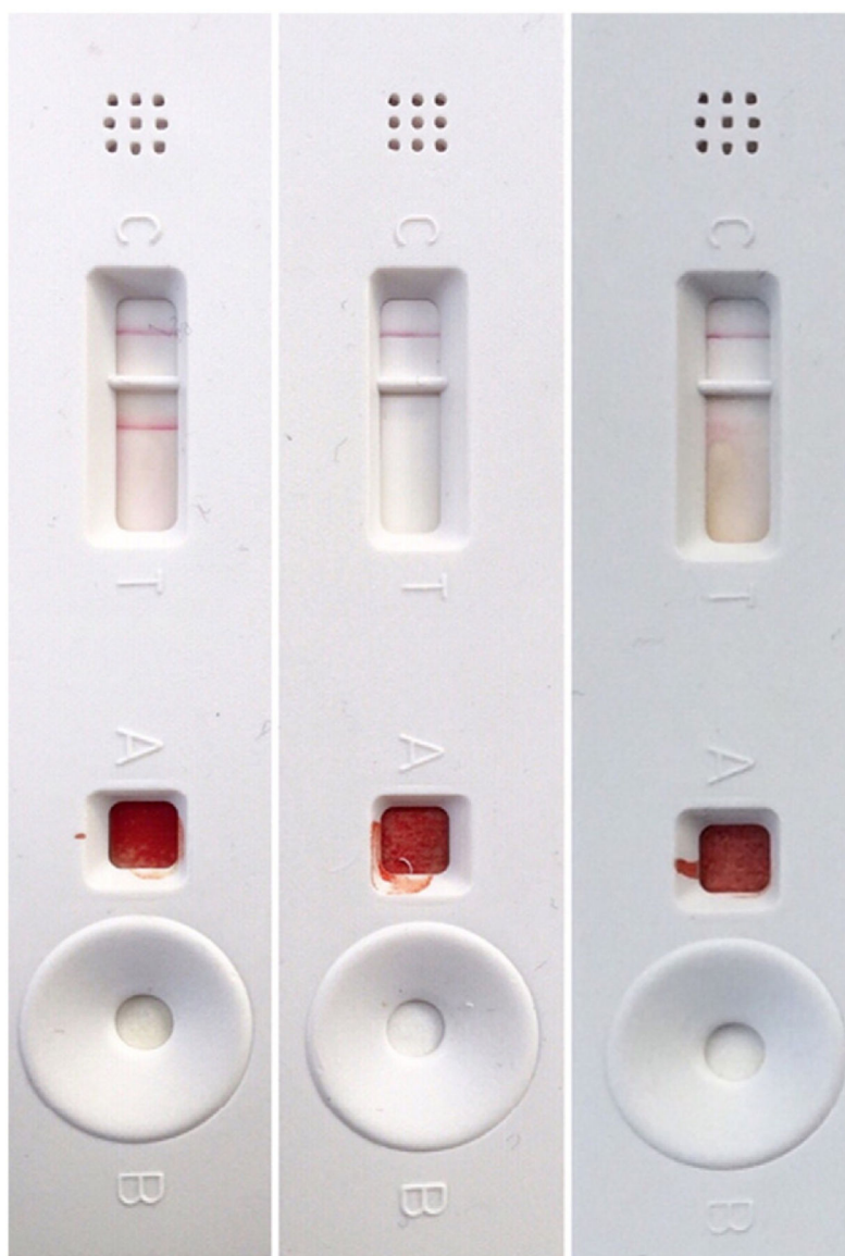
Fig. 1. Example of lateral flow assays graded as positive, negative, and equivocal (respectively, from left to right).
