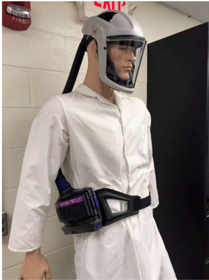
Figure 1. Loose-fitting PAPR with helmet. The belt-mounted air purifying unit is worn at the back during operation. Photo credit: NIOSH/NPPTL.
