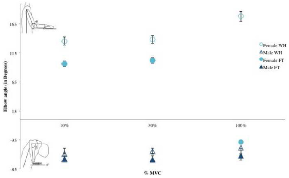
Figure 5. Comparison of elbow angles for female group (light blue) and male group (dark blue) pressing the plate in fingertip (FT) and whole hand (WH) postures at 0° pitch under 3 conditions (100, 30 and 10 %MVC).
