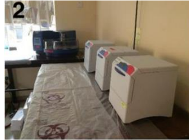
Room 2. The 96-well RNA extractor is in the center, 3 Bead Retrievers are on the right. Foil was placed over the window to deflect the heat of the sun
