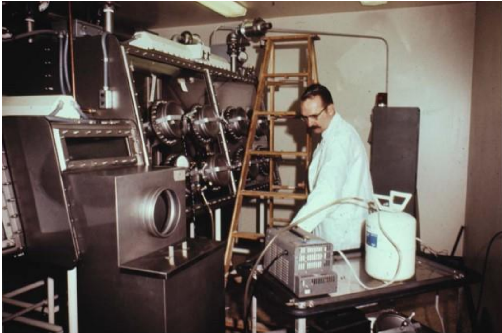
Bldg 8, Dr. Bob Huffaker, Biosafety Director, conducting a leak test on one of the glove box cabinets.
