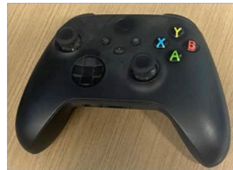
Xbox controller replacing manual cab controls
