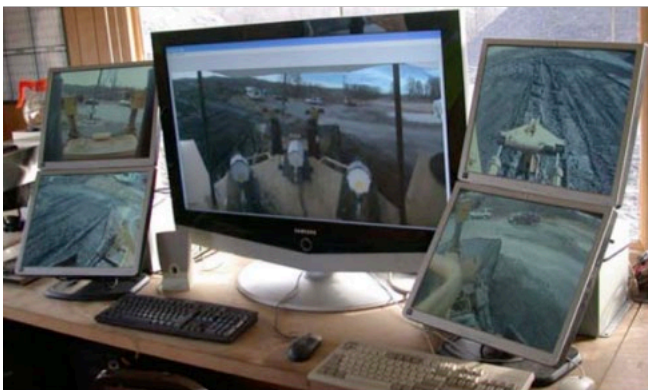
Figure 22: Video display arrangements suggested for remote stockpile dozer use by Schiffbauer et al (2007).
