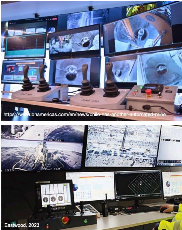
Figure 19: Joystick controls for automated drill rigs. Top: Anglo American IROC, Santiago, Chile. Bottom: Lake Vermont mine, Australia. (Eastwood, 2023)
