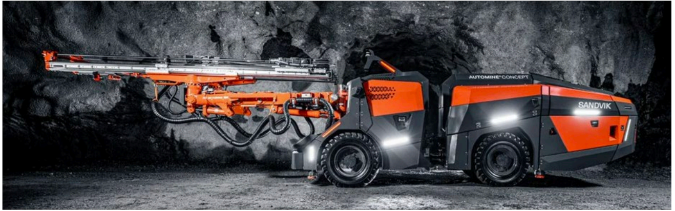
Figure 11: Fully autonomous Concept underground drill including autonomous tramming and drill-bit change (Butcher, 2023).
