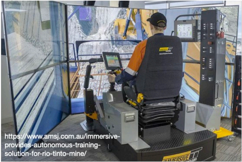
Figure 17: Virtual excavator simulator used for training operators to interact with autonomous haulage.
