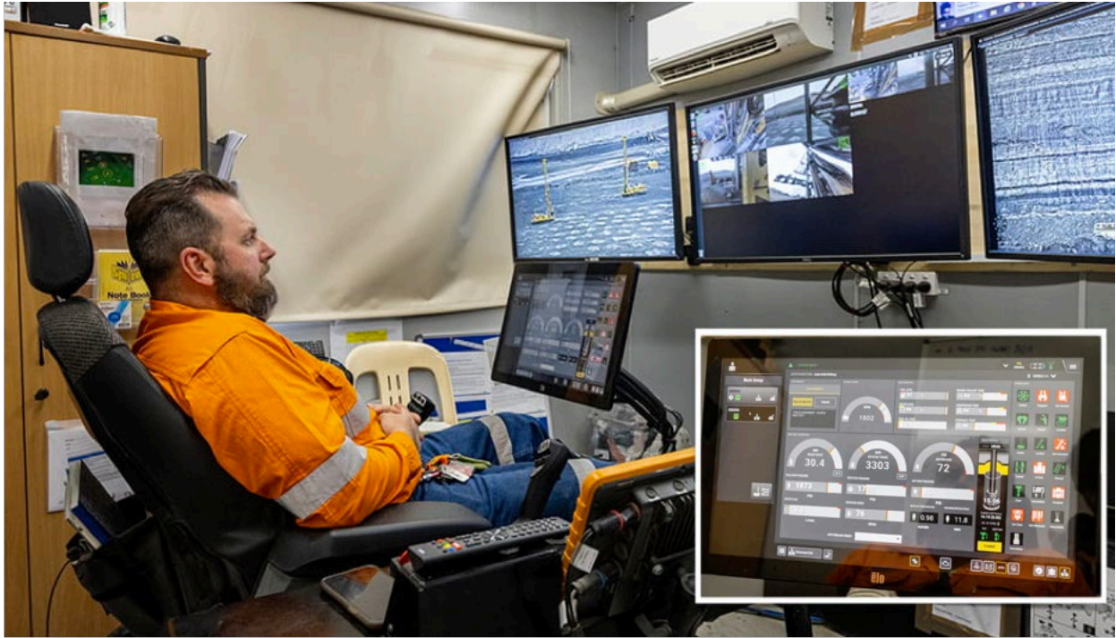
Figure 18: Replica drill cab workstation and interface for automated drill rig. (Westrac, 2022).
