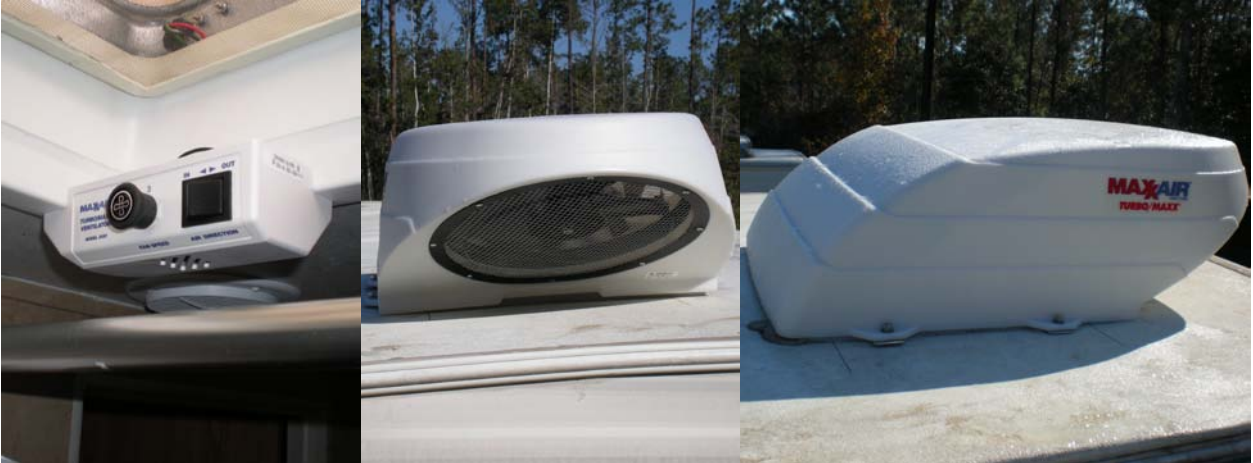
Figure B-10. MaxxAir unit installed in Trailer 9.
