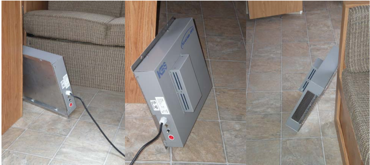
Figure B-6. KES/AiroCide unit placed in Trailer 6.
