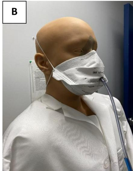
Fig. 2B. Medium Static Advanced Headform
