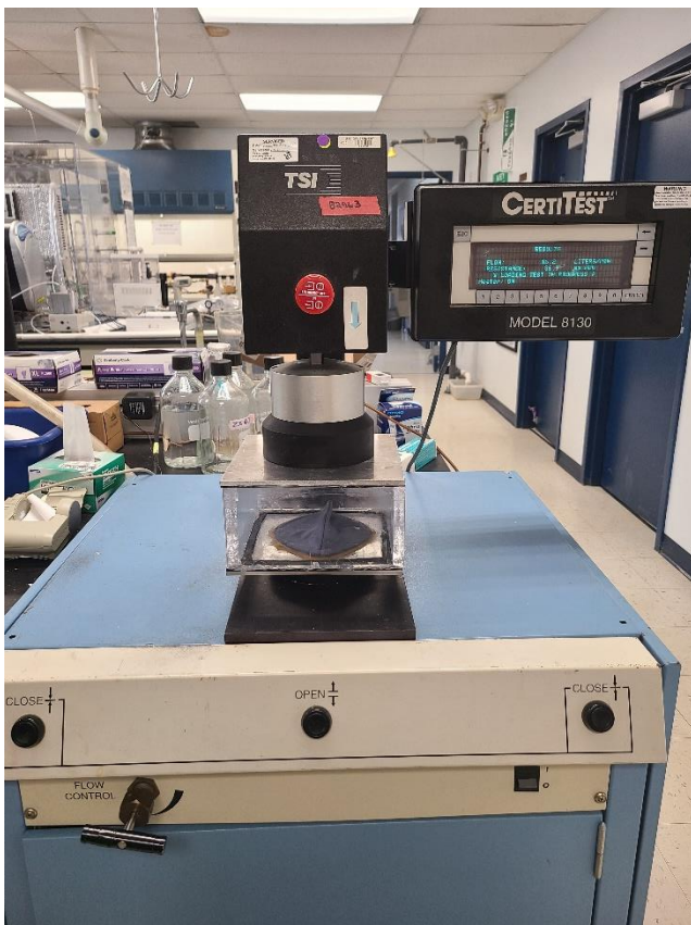
Figure 2: Laboratory Test Photos (TSI, Inc. 8130 filter tester)
