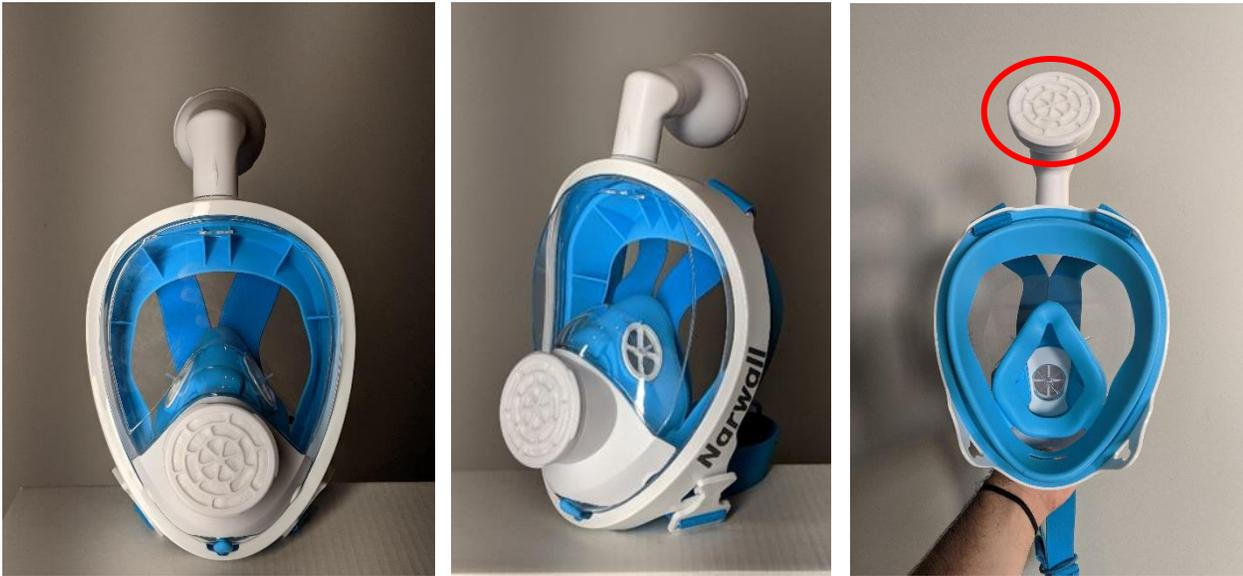
**Figure 1: Narwall Mask LLC front (left image), side (middle image) and interior (right image) views. The filter is shown in the red circle and was removed for filtration testing.**
