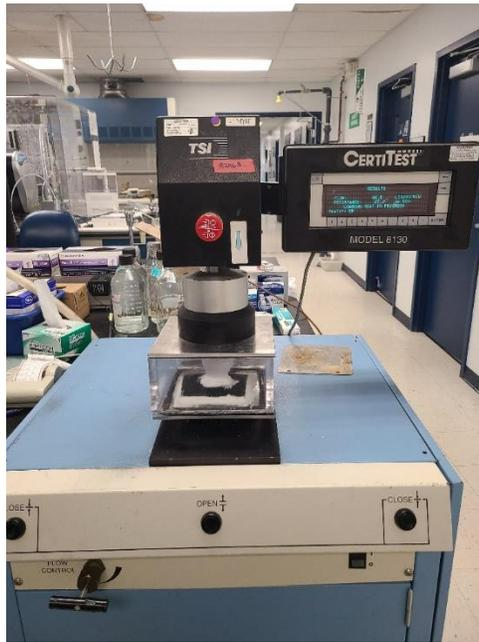
**Figure 2. Laboratory Test Photo (TSI, Inc. 8130 filter tester). Due to the design of this respirator, the filter housing was removed from the device and tested for filtration.**
