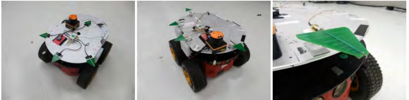
Figure 3: Proof of concept prototype. This platform was used to test the antenna diversity sensing system and the motion planning for communication coverage.
