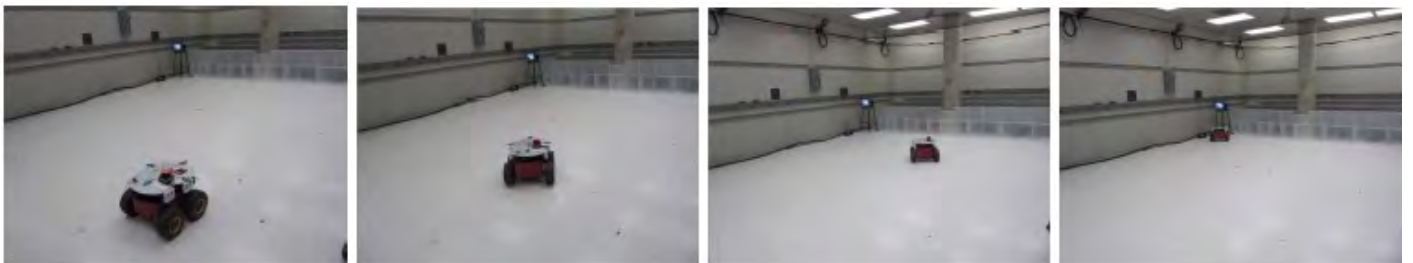
Figure 4: Motion sequence of the robot with the antenna array transceiver on top approaching the origin of the signal.
