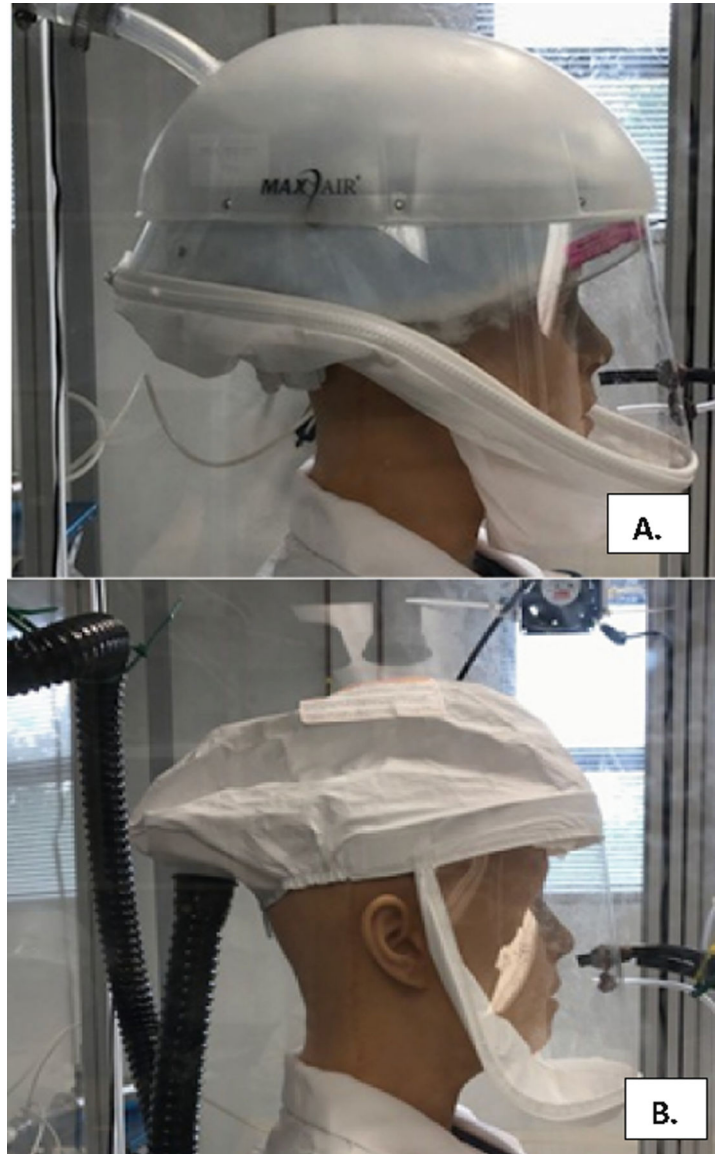
Fig. 1. PAPR models. (A) MaxAir ® 78SP-36 Cuff System with disposable cuff (size S/M) (Bio-Medical Devices, Inc., Irvine, CA); (B) 3M Air-Mate ™ with BE-12 facepiece (size regular) (3M Company, St. Paul, MN)
