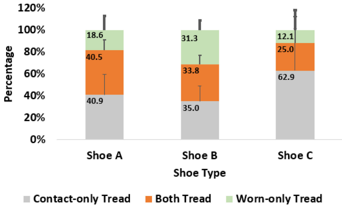
Figure 5: Stacked column plot showing proportions of treads that were in contact with the ground and were worn (middle bar, “Both Tread”), not in contact but were worn (top bar, “Worn-only Tread”), and in contact but were not worn (bottom bar, “Contact-only tread”). Data values indicate mean value across participants within shoe type, and error bars indicate standard deviation.
