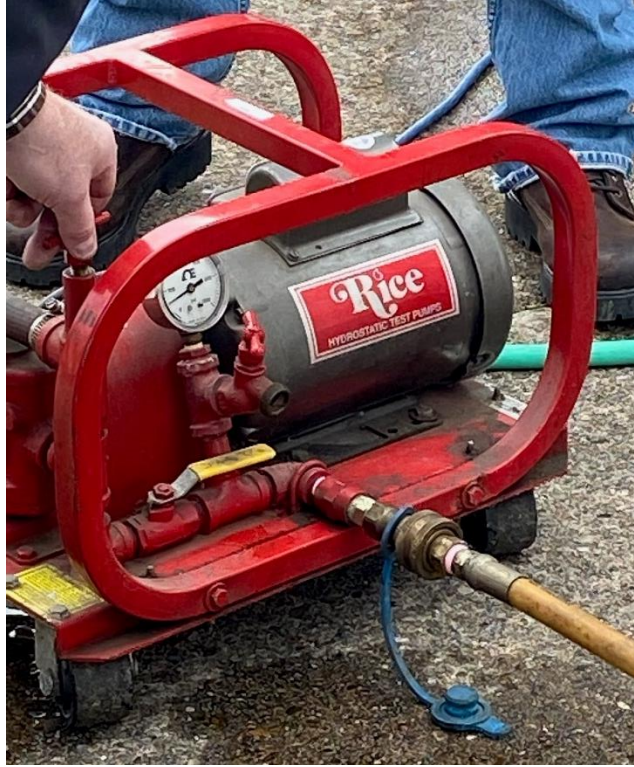
Figure 129 - Hydrostatic Test Pump
