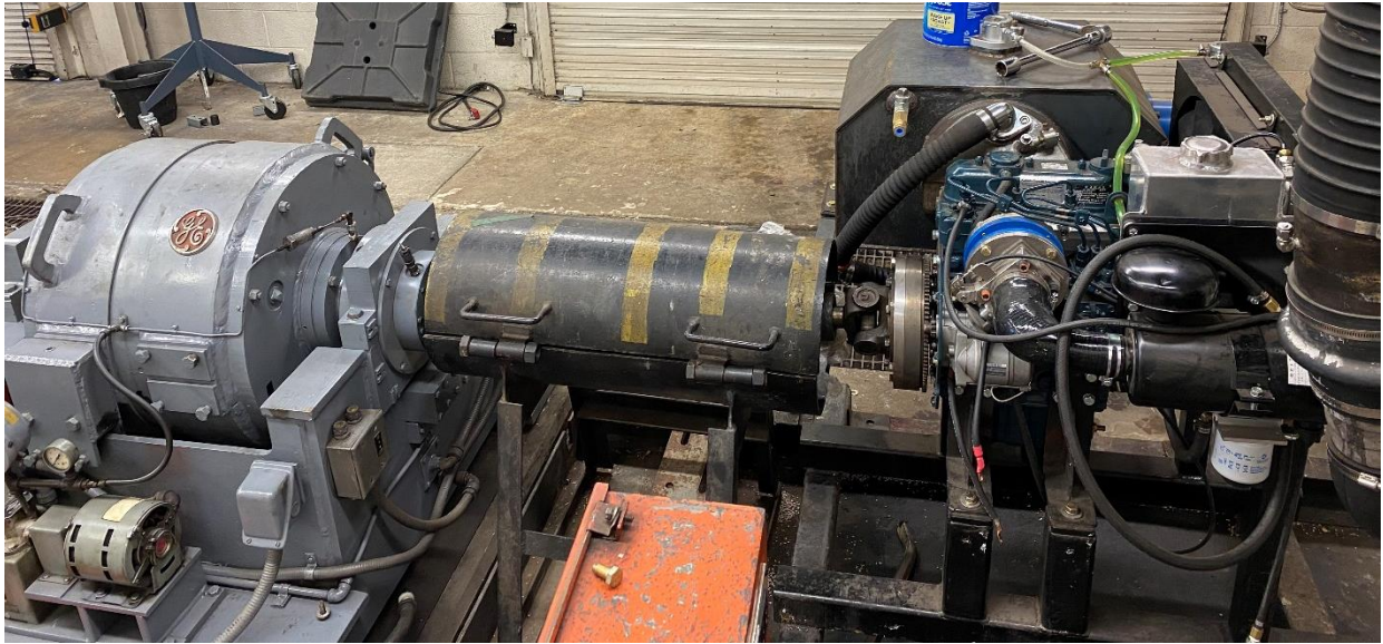
Figure 138 - Test Engine Dynamometer Installation
