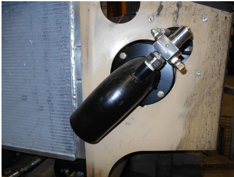
Figure 37 - Exhaust Outlet and Temperature Sensor
