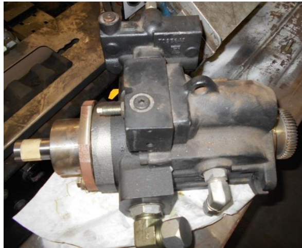
Figure 74 - Hydraulic Pump with Auxiliary Drive
