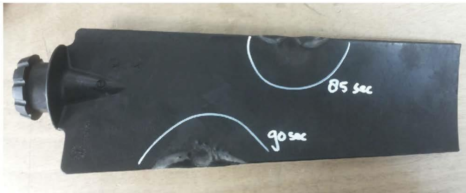
Figure 4: 4Z blade with times to extinction
