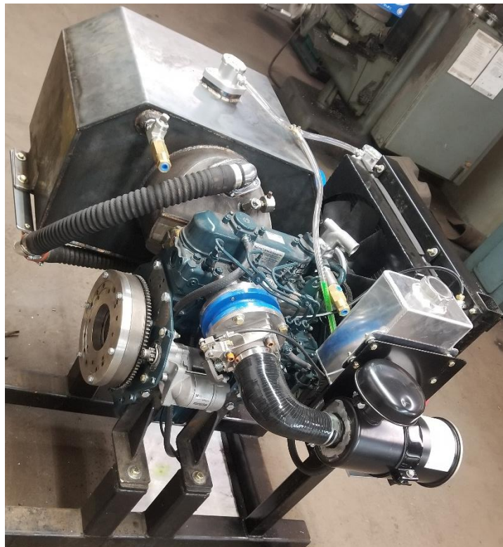
Figure 124 – Air Intake Side of Test Engine Assembly
