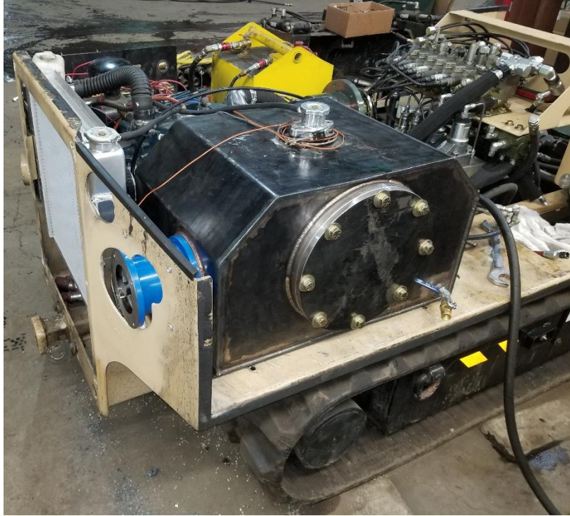
Figure 36 – Exhaust System on Machine for Initial Start Test
