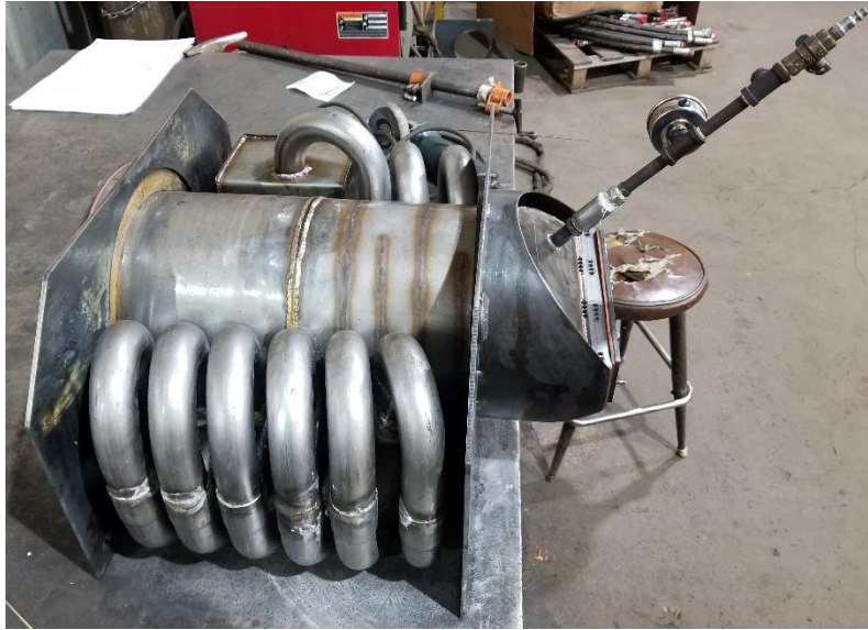
Figure 63 - Exhaust Cooler Fabrication
