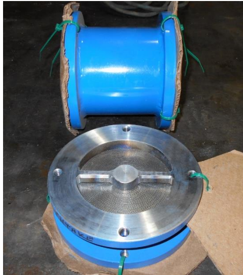
Figure 30 - Intake and Exhaust Flame Arrestors
