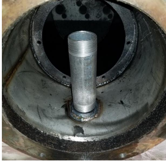
Figure 20 - Exhaust Box Riser Pipe Modification
