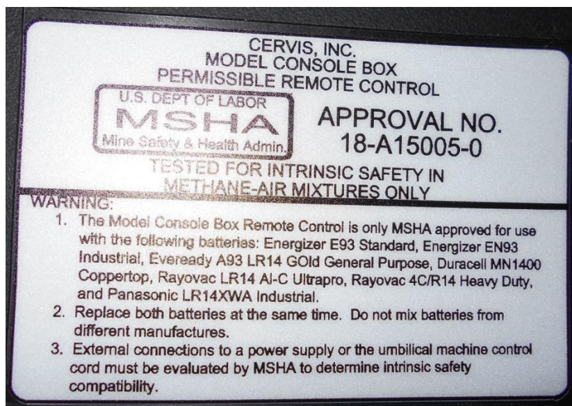
Figure 81 - Radio Transmitter Approval Tag
