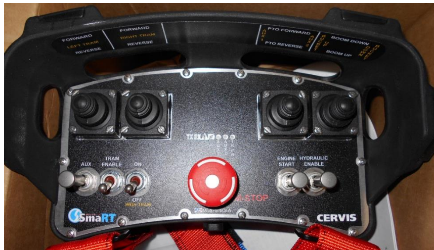
Figure 80 - Permissible Radio Transmitter
