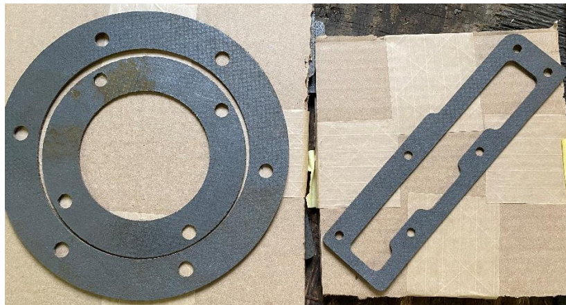
Figure 132-Exhaust and Intake Gaskets
