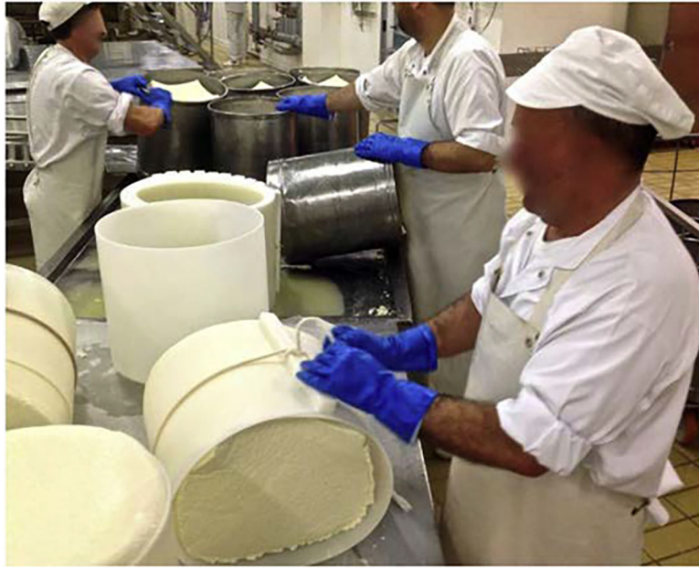
Fig. 3. An example of a cheese processing station consisting of three subtasks: turning, tightening and tying plastic mold covers around the cheese.
