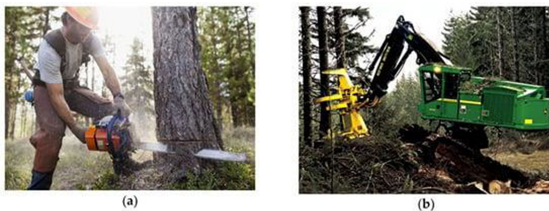
Figure 1. The primary logging systems for felling trees: (a) conventional chainsaw felling and (b) heavy mechanical equipment felling using a feller-buncher.
