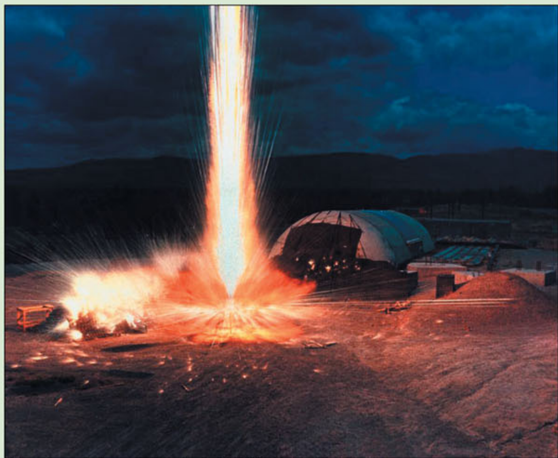
Fig. 2. An explosive testing “shot” at the PHERMEX facility, TA-15
