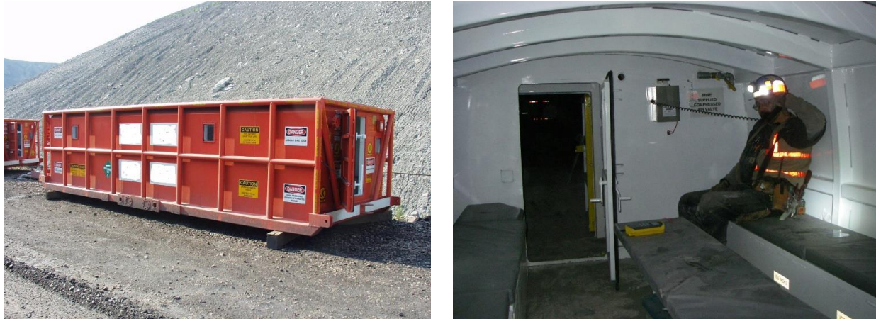
Figure 21. External view of a portable rigid RA (left) and internal view of a portable rigid RA (right).
