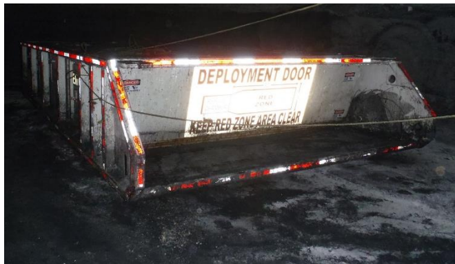
Figure 20. Non-deployed portable tent-type RA being moved in an underground coal mine (left) and a deployed portable tent-type RA in a warehouse facility (right).
