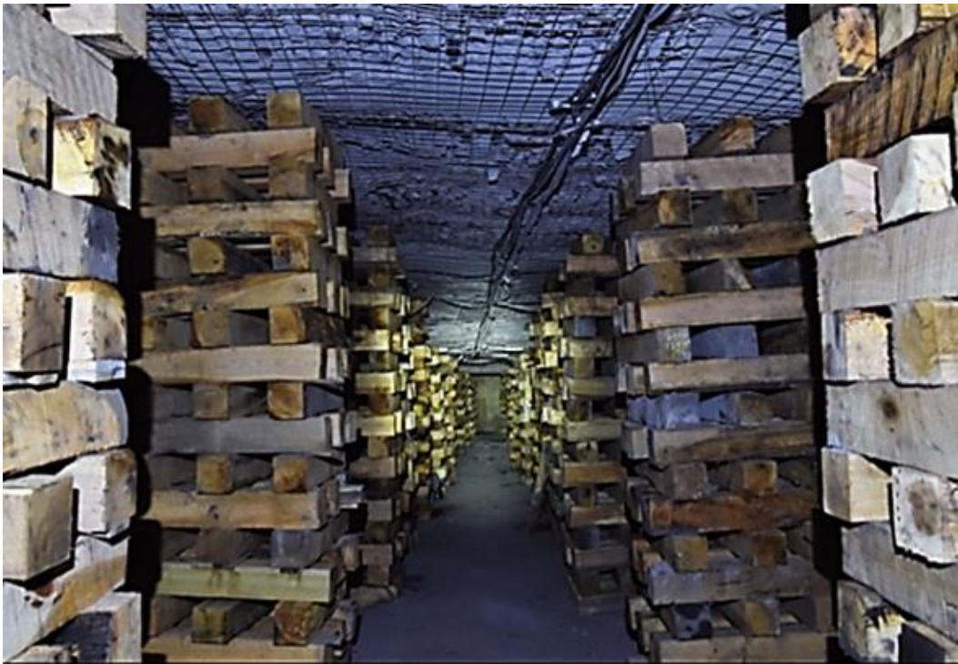
Figure 42. Coal mine entry with standing supports installed, including cribs, roof bolts, steel straps, cable bolts, and roof screen.
