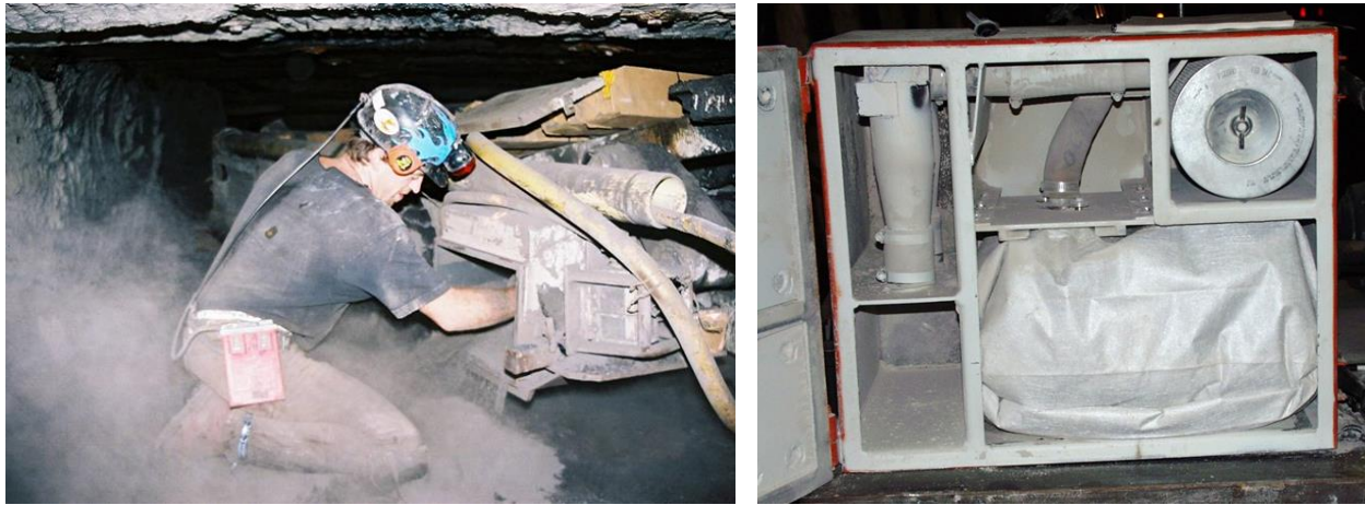
Figure 59. Miner cleaning collector box (left) and collector bag containing dust (right).
