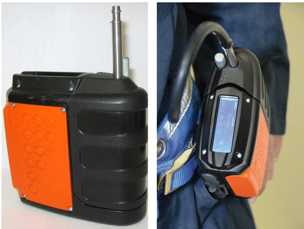
Figure 72. Airtec diesel sampler (left) and being worn on a miner's belt (right).
