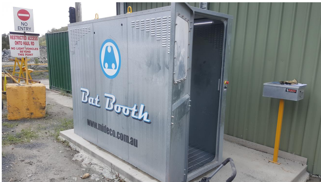
Figure 67. A clothes cleaning booth based on NIOSH-developed technology located in Narangba, Australia, at a thoroughfare between the quarry and workshop.
