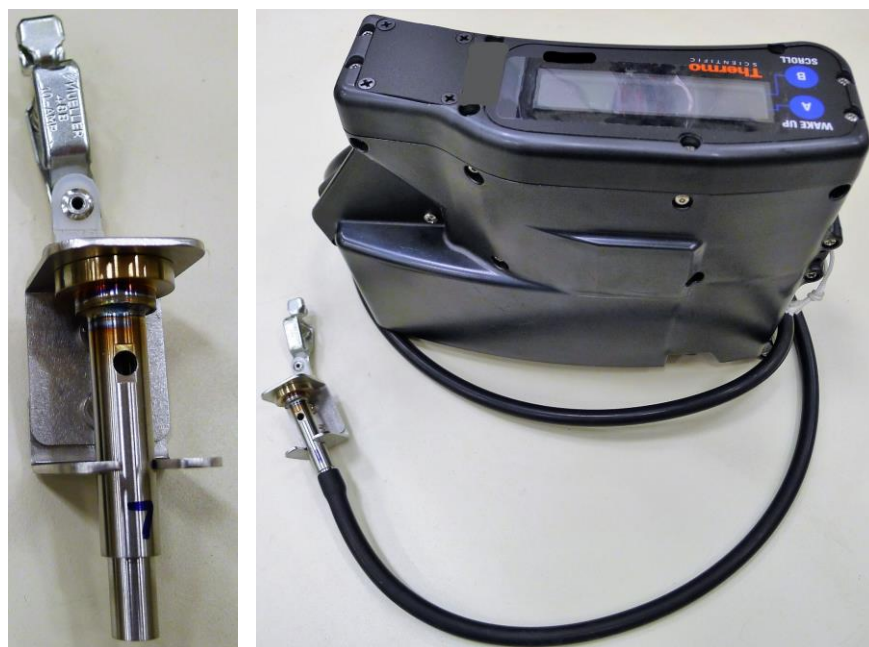
Figure 57. New inlet design (left) and PDM3700 (right).
