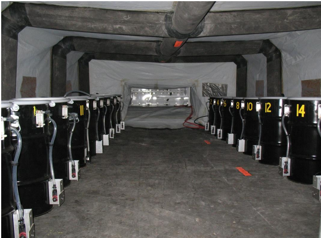
Figure 24. Underground heat and humidity testing with simulated miners in a tent-type RA in NIOSH's Experimental Mine.
