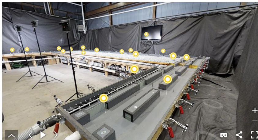
Figure 7. Screenshot of the LIAM, which provides an online virtual tour of varying ventilation configurations . When clicked, each yellow circle offers detailed ventilation information specific to that area of the model.
