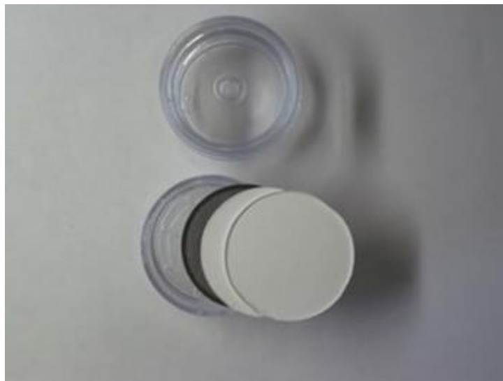
Figure 75. Two filters in tandem and a stainless steel backing pad to be inserted into a standard three-piece cassette.
