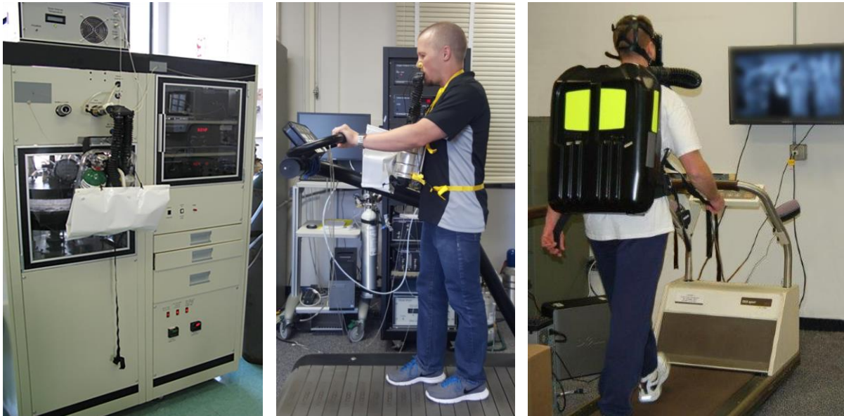
Figure 8. Equipment used to test CCERs in the ABMS Lab (left). Human subject testing in the ABMS Lab of an SCSR (center) and a CCER (right)
