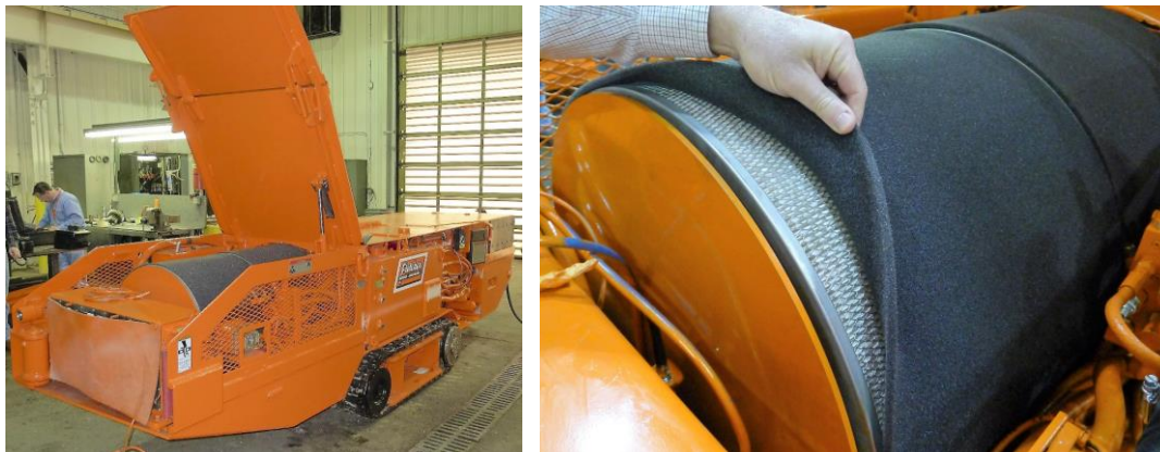
Figure 61. Mobile dry scrubber (left) and filter cartridges (right).
