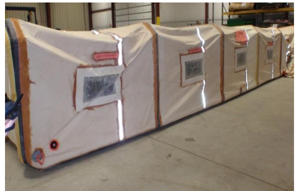
Figure 20. Non-deployed portable tent-type RA being moved in an underground coal mine (left) and a deployed portable tent-type RA in a warehouse facility (right).
