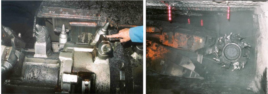
Figure 62. Spray nozzle located behind cutting bit (left) on wet-head continuous miner (right).
