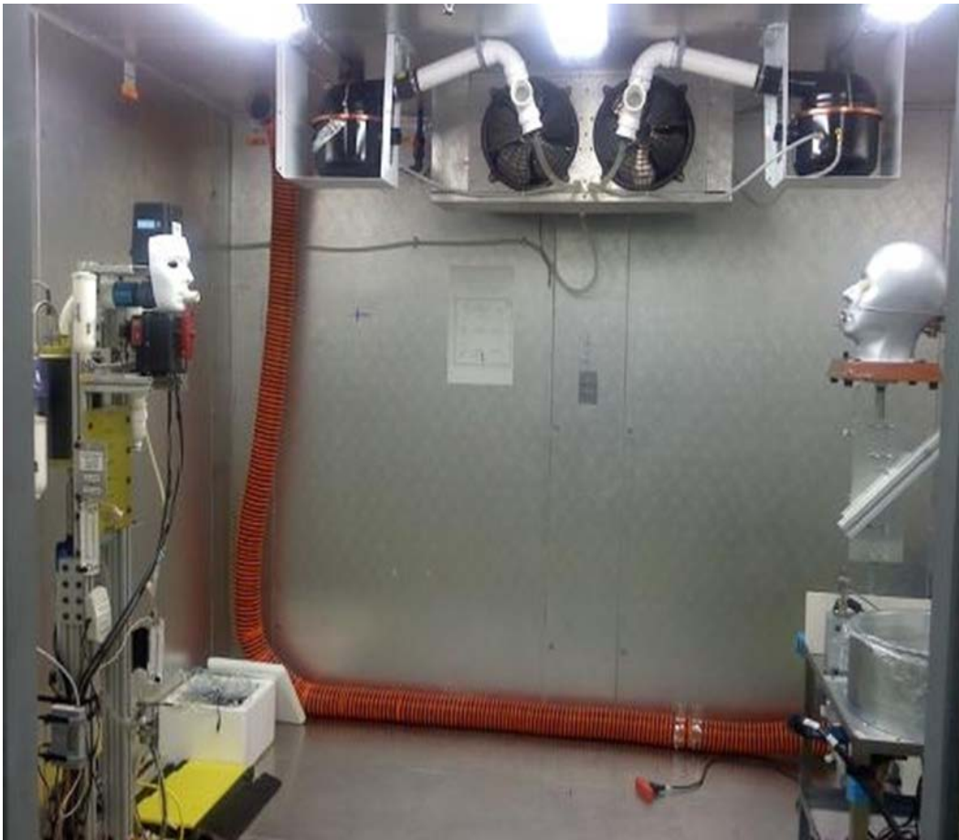
Figure 35. A simulated examination room with coughing (left) and breathing simulators (right) to study the behavior of airborne influenza virus. [Photo credit: NIOSH]
