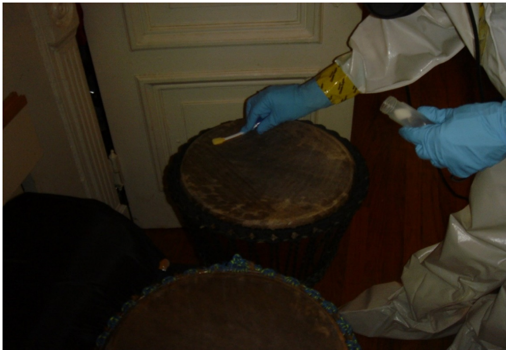
Figure 13. NIOSH Responder sampling drum head as part of the 2006 New York anthrax response. [Photo credit: NIOSH]
