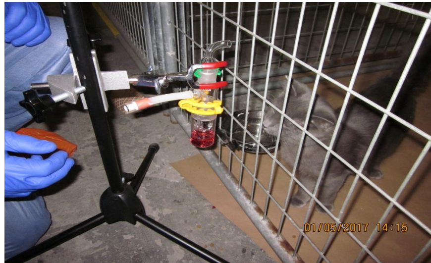
Figure 37. NIOSH staff collecting air sample looking at potential aerosol transmission during care of cats infected with avian influenza. [Photo credit: NIOSH]
