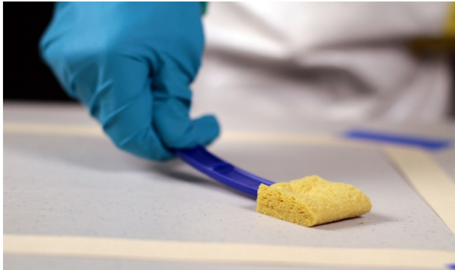
Figure 14. Example of a cellulose sponge for collecting a B. anthracis sample. [Photo credit: NIOSH]
