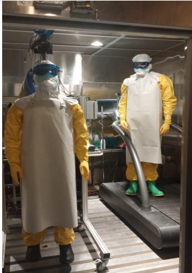
Figure 32. NIOSH PPE research looking at heat stress using manikins. [Photo credit: NIOSH]
